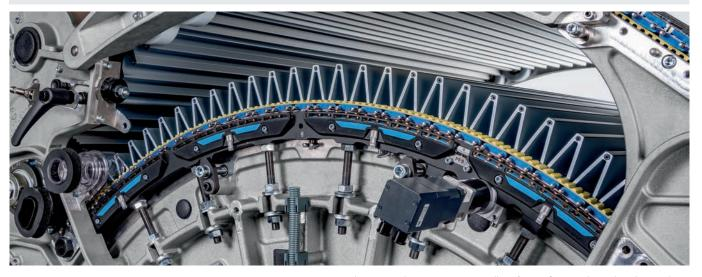
The TC 19i with T-GO gap optimizer allows for significant quality and productivity leaps which reduce the energy demand per kilogram of card sliver
